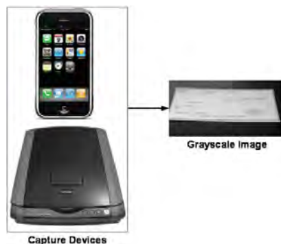
Figure 3—Flatbed scanners and cell phones only capture images and not MICR data
