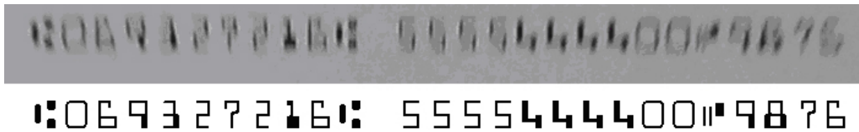
Figure 4— MICR line from RDCC captured check image before and after processing
