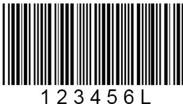
Figure 2 - A Typical Bar Code Symbol in the Code 39 Symbology
