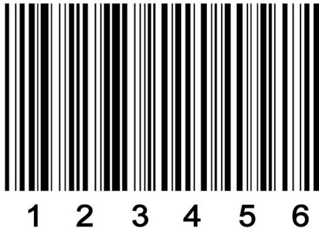
Figure 5- A Bar Code With Checksum Character
