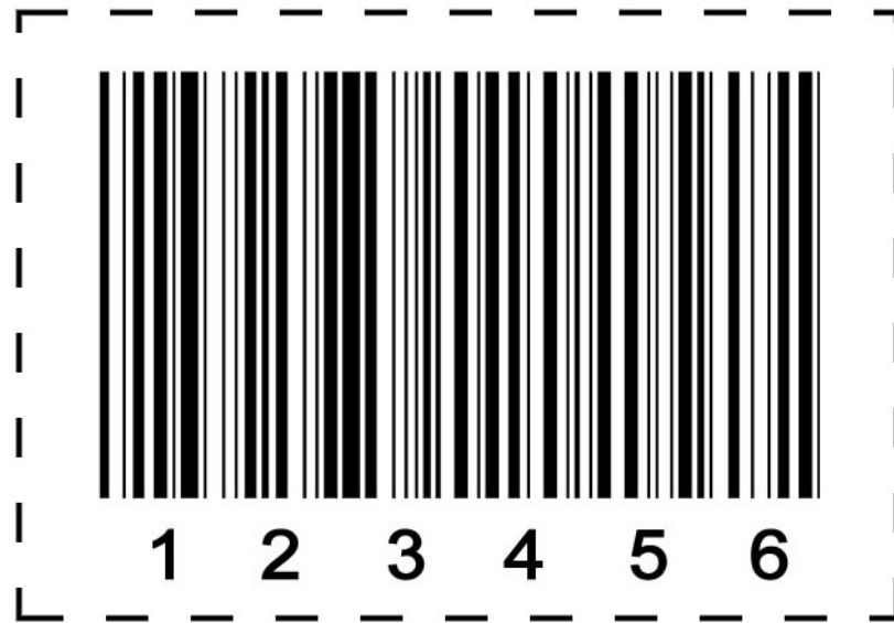
Figure 4 - A bar code with quiet zones on four sides
