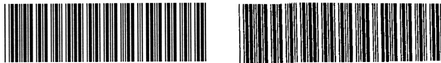
Figure 12 - A Bar Code Before and After Faxing
