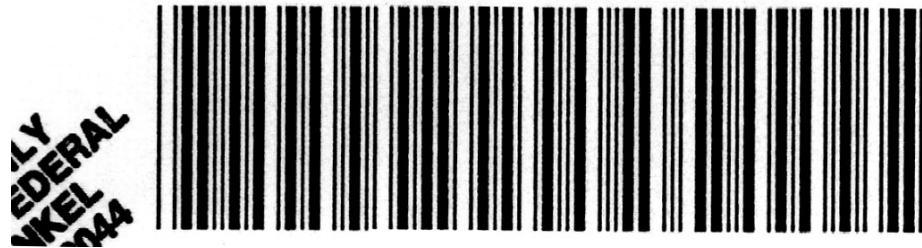
Figure 10 - Bar Code With Quiet Zone Violation
